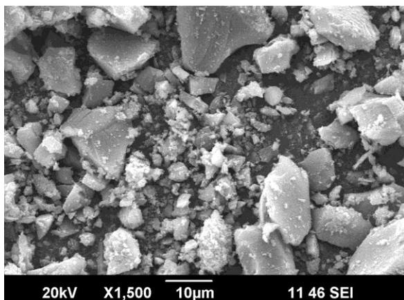
Fig 4. SEM micrograph of the as prepared calcinated TiO<sub>2</sub>Nanoparticles.
