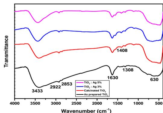
Fig 2. FTIR spectrum of the as prepared and Ag-doped TiO<sub>2</sub> Nanoparticles.
