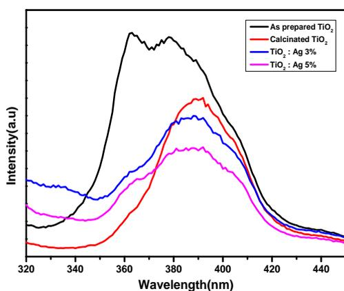
Fig 9. Photoluminescence spectrum of the as prepared and Ag-doped TiO<sub>2</sub> Nanoparticles.
