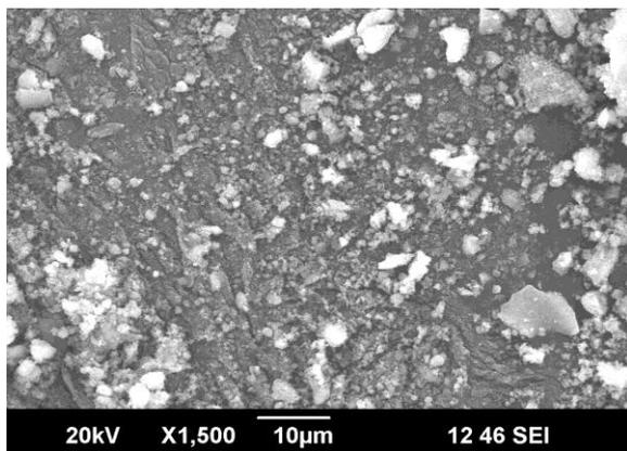
Fig 6. SEM micrograph of the 5 wt% Ag-doped TiO<sub>2</sub>Nanoparticles.
