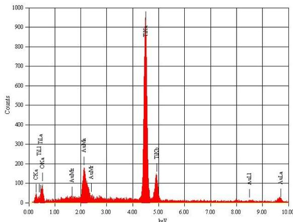
Fig 7. EDS spectra of the as prepared TiO<sub>2</sub>Nanoparticles.
