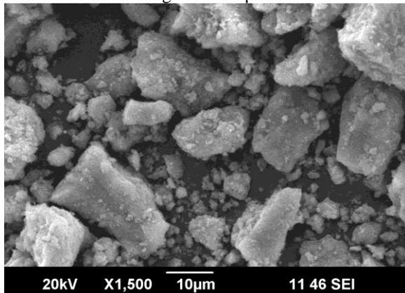
Fig 5. SEM micrograph of the 3 wt% Ag-doped TiO<sub>2</sub>Nanoparticles.
