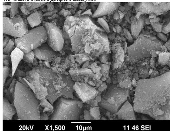
Fig 3. SEM micrograph of the as prepared TiO<sub>2</sub> Nanoparticles.
