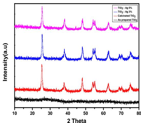
Fig 1. Powder XRD spectrum of the as prepared and Ag-doped TiO<sub>2</sub> Nanoparticles.
