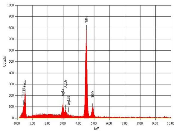
Fig 8. EDS spectra of the Ag-doped TiO<sub>2</sub>Nanoparticles.
